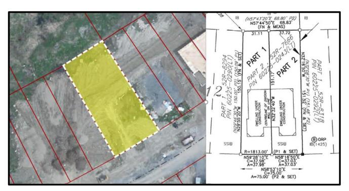
This approach is used because of the difficulty the builder would have in ensuring that the common center wall between the two dwelling units was constructed exactly on the property line. The foundation walls are in place and a reference plan has been submitted. The accurate legal descriptions are determined for the property and the individual lot(s) can subsequently be sold.
